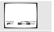
4 Move the cursor control joystick up or down to select the setting to adjust.
